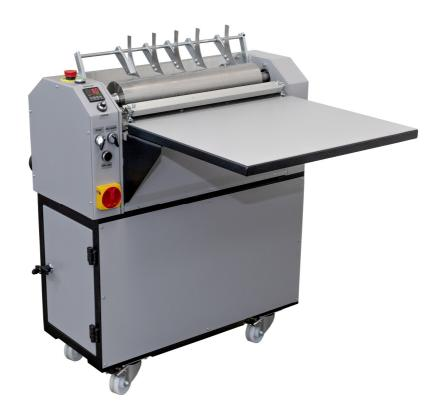
Used for application of thin layer of glue on flat surfaces like paper, eco leather, pvc etc.
