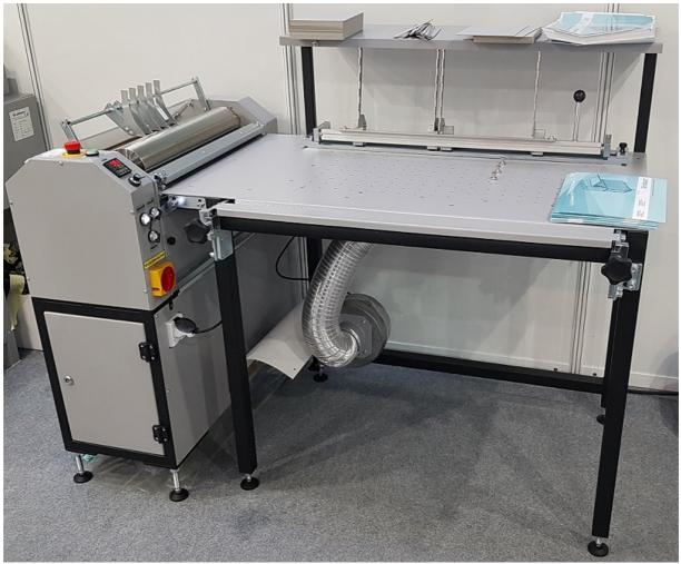
Set consist of gluing machine GM-520 and casemaker.
