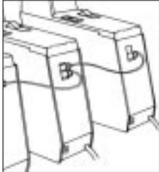
Serial mounting via opto cables for greater production capacity.
